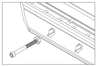
For rail mounting of the Benchrest Forearm Adapter, position the hex nuts using the bolt as shown.
