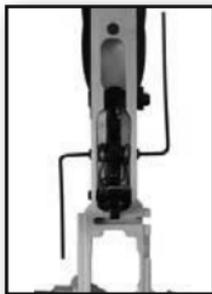
Apply a very small amount of thread locker to the two remaining 6-32 x 3/16" buttonhead cap screws and install them tightly into each of the anti-walk pins. Use the two 1/16" hex key provided to firmly tighten the screws into the threaded holes of the pins.
