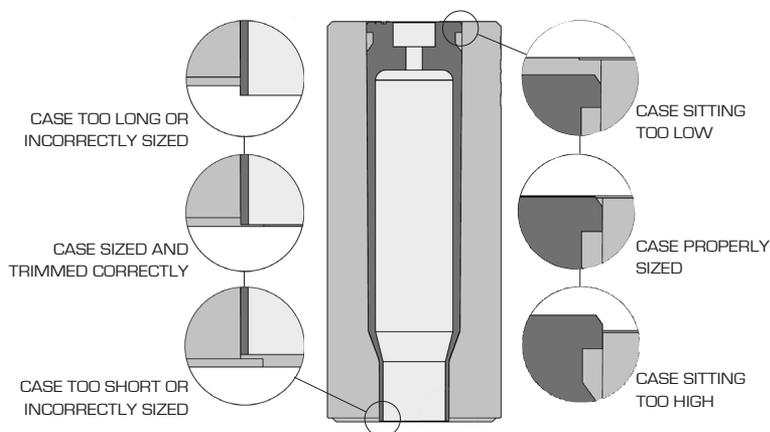
You can also verify headspace by checking protrusion on the bullet end when the gauge is stood upright on the case rim end on a flat surface. Here, the lip of the cartridge should come to rest between the outer rim and central channel. If it does not, it is either too long/short or sized incorrectly.
