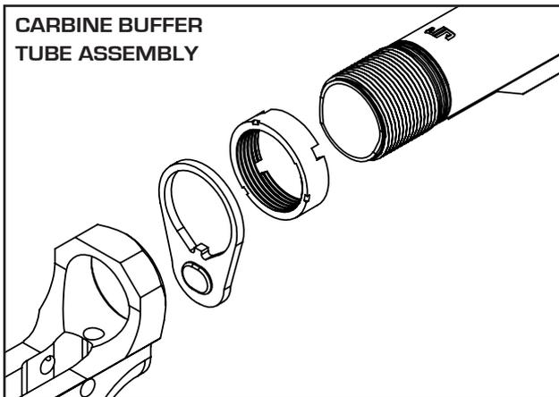
5. Hand tighten the castle nut against the end plate, which will butt up against the rear of the receiver.
