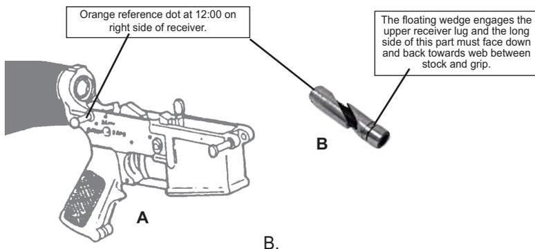
Now using the provided allen key, tension the device and if it is properly installed, the upper assembly will be pulled back and down on the lower with no remain-
