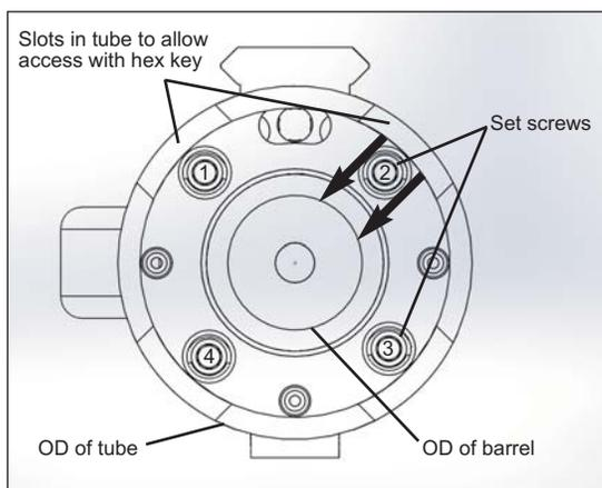
12. Determine whether the barrel is centered by examining the distance between the barrel and the inner wall of the Hand Guard Tube. If not, use the Jam Nut to center the barrel by tightening the screws accordingly. For example, tightening set screw 2 indicated at left will move the inner edge of the tube towards the barrel as shown by the arrows. This same principle applies to each of the set screws, which together allow for proper alignment.
