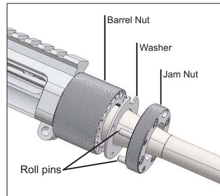
9. Thread the Hand Guard Tube onto the Jam Nut and continue to thread it down onto the Barrel Nut. Use caution when transitioning from the Jam Nut to the Barrel Nut to avoid cross-threading the Barrel Nut and the Hand Guard Tube. Try to keep the Jam Nut, Washer and Barrel Nut all together and touching when crossing over. The clocking threads will determine exactly how much space will be in between the nuts and the washer, but it should not exceed the thread spacing.
