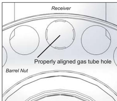
5. Install the Barrel Nut using a wrench to partially tighten and loosen the nut 3-4 times to seat the barrel. On the last tightening, torque the Barrel Nut to 40-80 foot-pounds. Verify that the gas tube hole in the receiver is aligned with one of the holes in the Barrel Nut.
