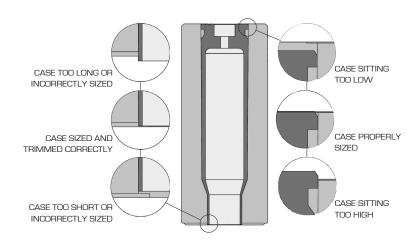
You can also verify headspace by checking protrusion on the bullet end when the gauge is stood upright on the case rim end on a flat surface. Here, the lip of the cartridge should come to rest between the outer rim and central channel. If it does not, it is either too long/short or sized incorrectly.
